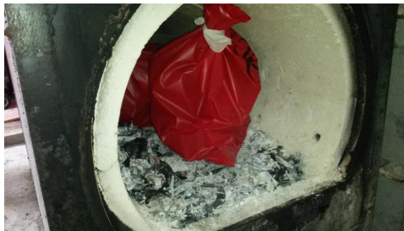
Photo B: Red plastic bag not adequately sealed & Incinerator not cleared/cleaned of ash & residuals (SOURCE: Auditor Walkthrough - April 3, 2017)
